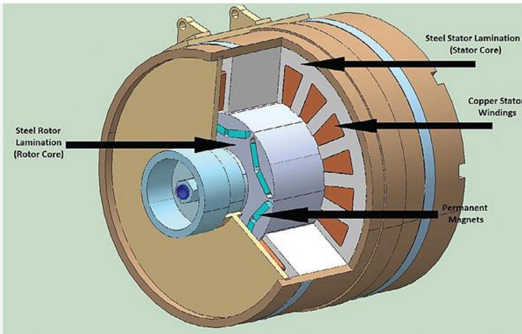
The parts of a permanent magnet AC motor. The rotor construction is similar to an induction motor but here the aluminum or copper inserts are replaced with permanent magnets. *Image by: MagNet from Infolytica Corp.*
