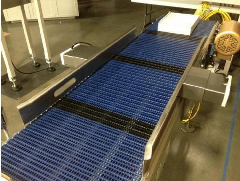
The pneumatic-based Compact Anysize positioning system for packaging conveyor lines frees food and beverage plants from having to make time-consuming manual adjustments when changing over a packaging line to accommodate different bottle, package, or case sizes.
