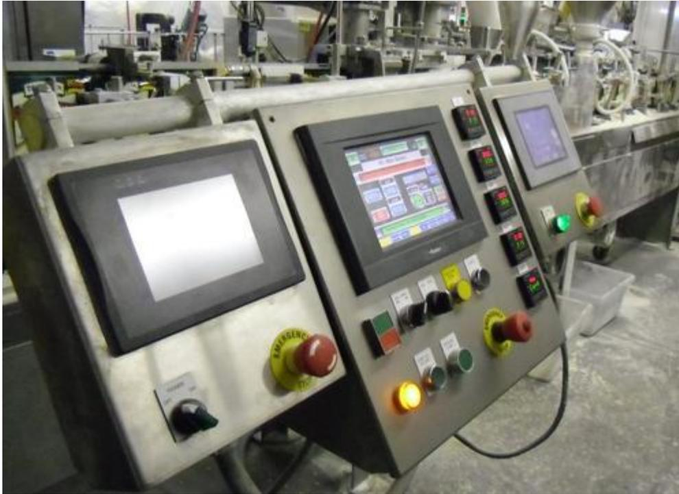
Xpress HMI is being used on a packaging machine in a food processing plant.
