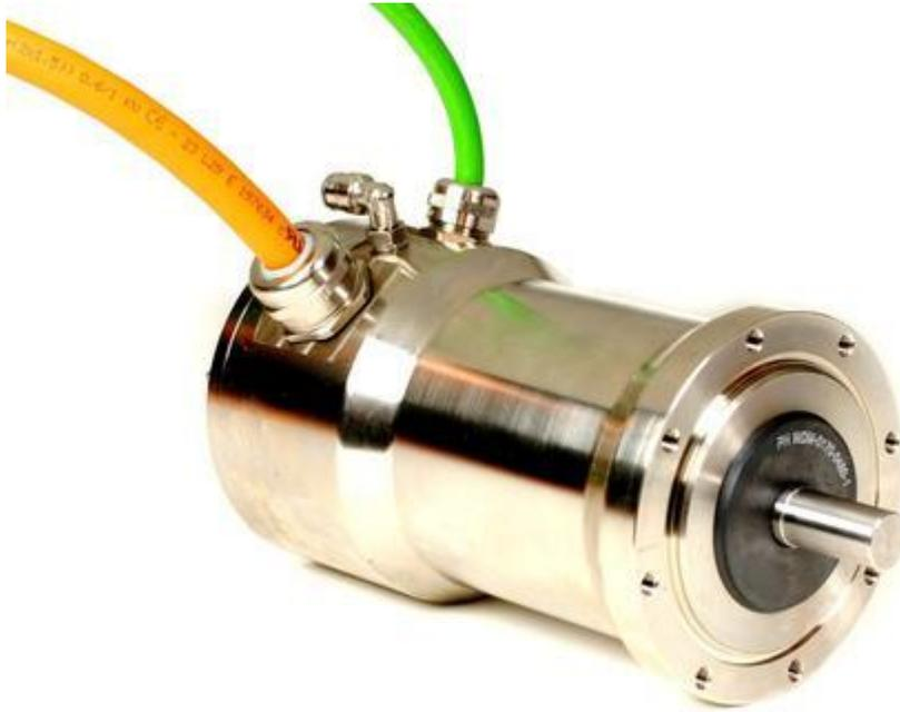
The MPW stainless-steel servo motor is designed for clean-in-place, high-pressure, highly caustic washdown settings such as those found in the food and beverage industry. The motor features segmented core technology, which can yield 40% higher torque per unit size than conventionally wound servo motors.
