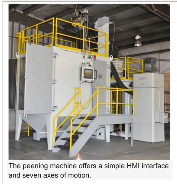
The peening machine offers a simple HMI interface and seven axes of motion.
