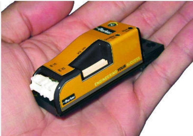
*This miniature stepper drive from Parker measures 1" x 1" x 3", runs on 24 VDC and is powerful enough to run a NEMA 17 stepper motor.*
