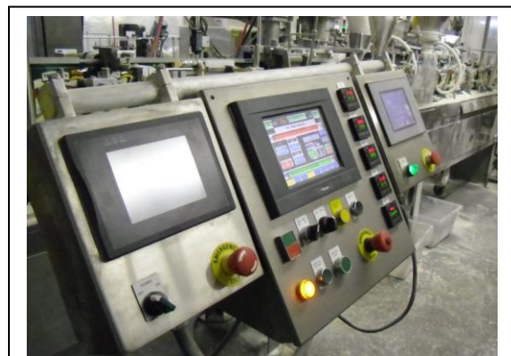
Here, the Crest horizontal packager wraps food according to commands programmed by the HMI. Displayed on the HMI is Interact Xpress software, which lets Crest revise and reuse applications.
