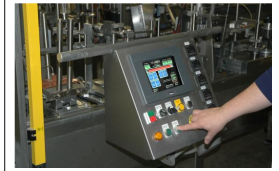
Here, the Crest horizontal packager wraps food according to commands programmed by the HMI. Displayed on the HMI is Interact Xpress software, which lets Crest revise and reuse applications.
